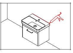
6 Once the basin is fitted and secured to the furniture unit, add a thin bead of silicone along with edge of the back of the basin.
