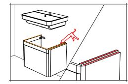
5. Having finishes all the plumbing connections, secure the basin to the unit using a silicone sealant. Make sure the basin is correctly aligned with the furniture and allow the sealant to dry. The silicone sealant will help the basin sit level on the furniture and protect the unit from water damage
