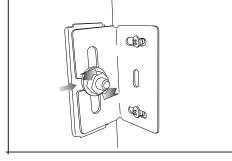
If the drawer needs drilling to install the handle: Ensure the paint does not blow on the front of the panels by placing the door (front face down) on a wooden board. Drill the pilot holes using an M4 drill bit. Fit the handles to the unit using the screws provided and a screw driver.
